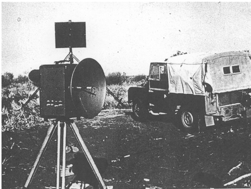
Figure 4 The Natmap MRA1 Tellurometer in South Australia in 1956
